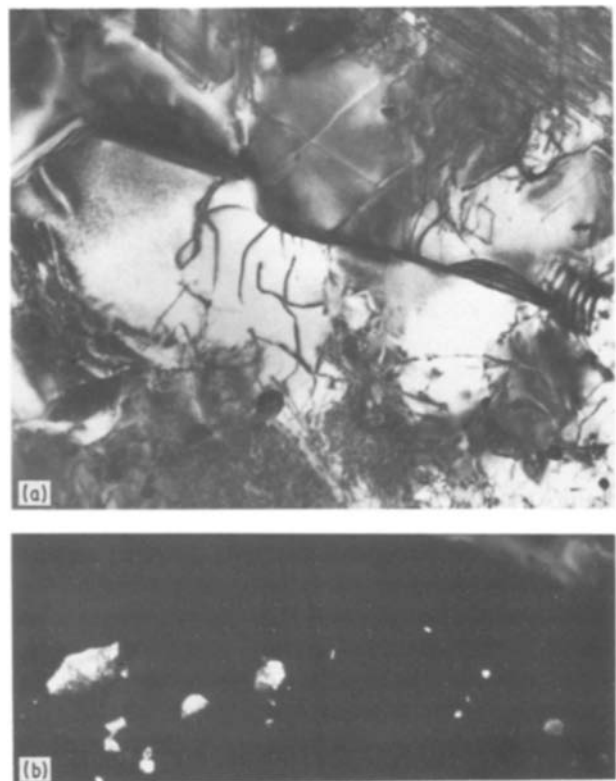
Figure 2 (a) A region containing typical low-dislocation-density regrown diamond, with a high-angle grain boundary crossing the field from above mid-height on left to below mid-height on right. Field width 2.6 \mu\text{m} , electron accelerating voltage 300 \text{ kV} . (b) Dark-field image, cobalt 200 reflection, of lower half of field in (a) showing cobalt inclusions strongly diffracting.
